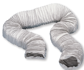
Class: M1 Minimum corvature radius: 0,6 \times \varnothing Operating temperature: -10^{\circ}\text{C} to +150^{\circ}\text{C}
