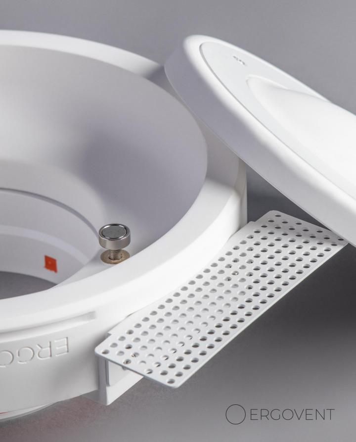
High quality, homogeneous gypsum body (without any drilling and gluing) 100 / 125 / 160 mm duct connectors with a double gasket Anti – vibration gasket between the body and the connector Side fasteners are easy to customize for any drywall thickness
