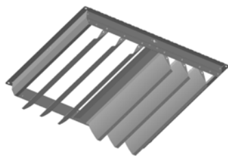
Fig. 18: Basic ceiling outlet
