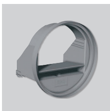
RD BP SM Auto-adjustable flow regulators. To be installed inside the cuff of the BDOP nozzles. 80mm diameter. Flow rate: 15 or 30 m 3 /h.
