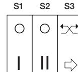
S3 switch activates the "Free cooling" (Bypass) mode, which stops alternate flow and keeps the fan in "extract-only" or "intake-only" mode, to avoid the heat exchange when necessary. To set the extract-only mode or intake-only, place the integral jumpers as per fig. 20A-20B). The front cover LED indicates when the Free cooling mode is on.
