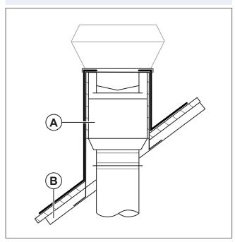
3 Install the duct and attach the product, with the installed FTG tilting device, on the top of the roof curb.
