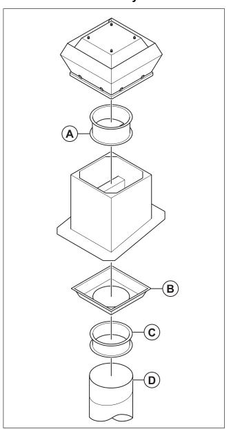
Systemair recommends to connect the duct (D) to a flexible connection (C), an inflow box (B) and a back draft damper (A).
