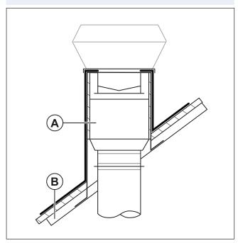
3 Install the duct and attach the product, with the installed FTG tilting device, on the top of the roof curb.
