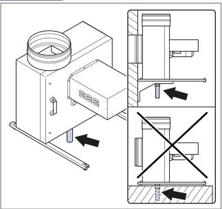
2 If wall brackets are used, install the wall brackets.
